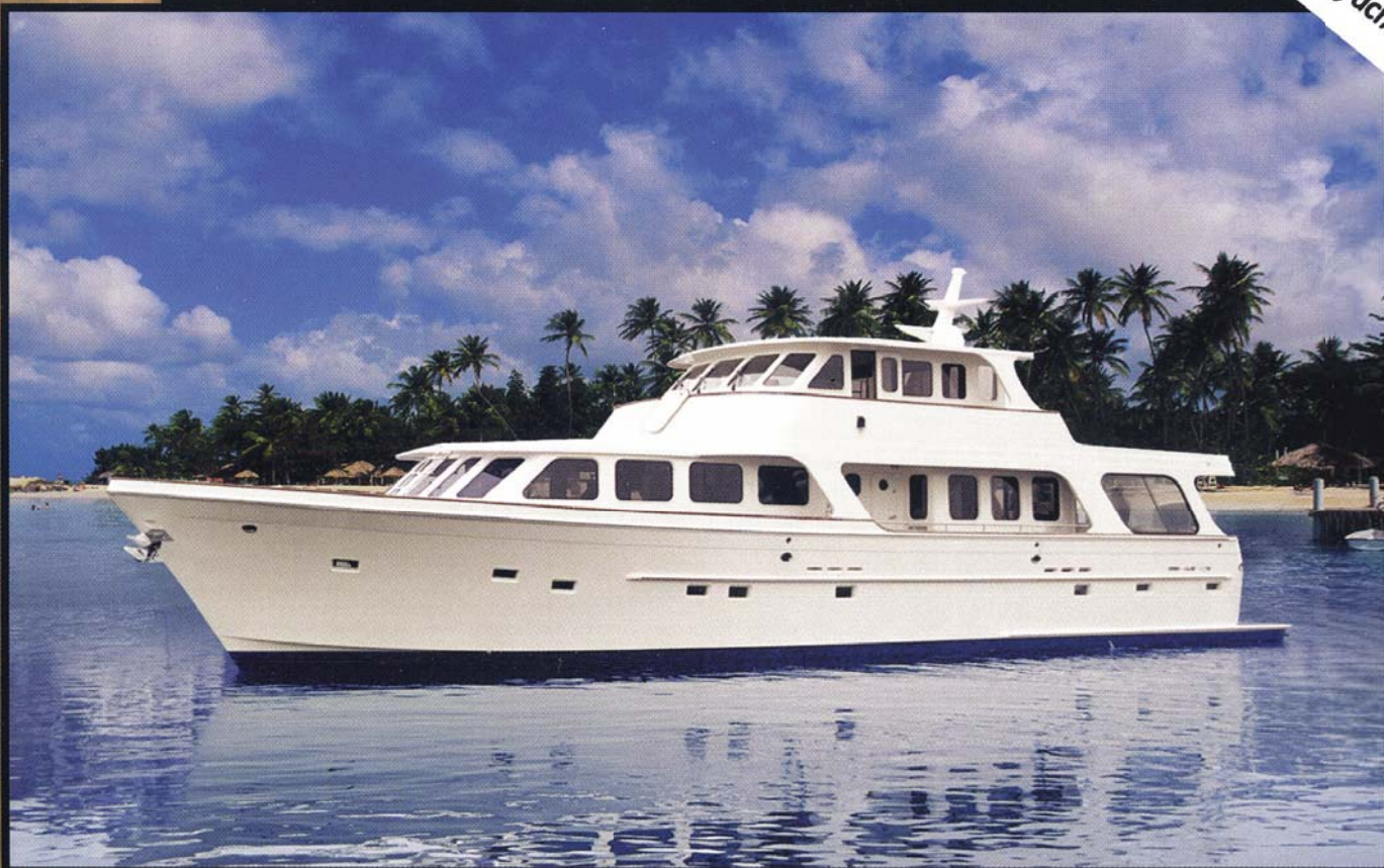
One nice touch on the Offshore 80 is her window frames, which are part of the mold for the fiberglass superstructure and, thus, won't corrode.
